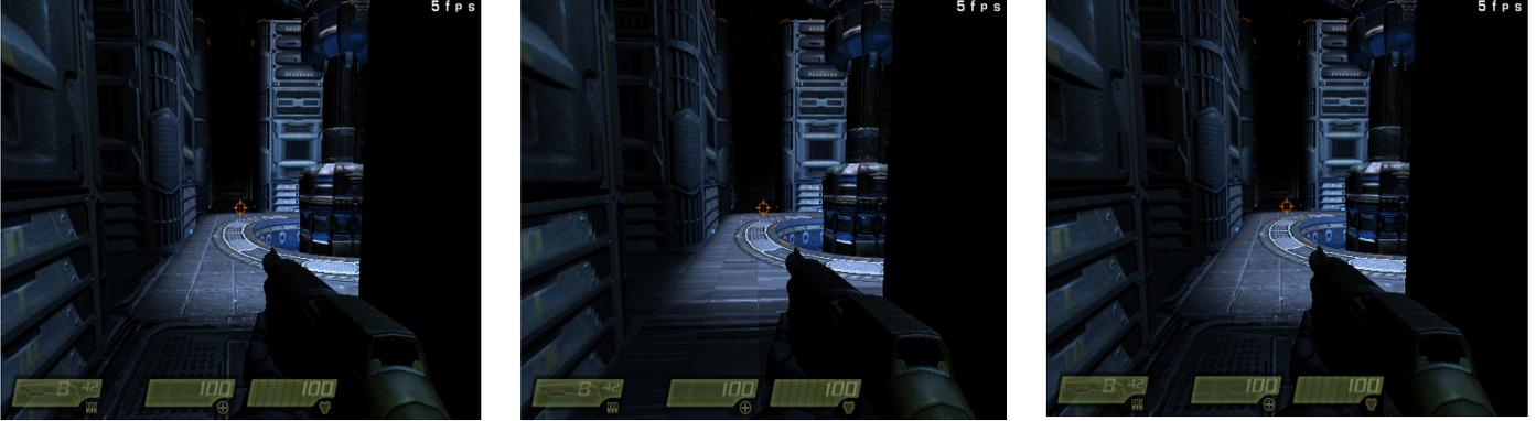
Fig. 3. Image in left is the reference frame produced by full-precision computations (32 bits) throughout the fragment shader. Image in the middle shows the result of reducing the precision of texture coordinates to 16 bits. Image in right shows the result of reducing the precision of color computations to 16 bits. There are no perceptible differences in the latter case.
