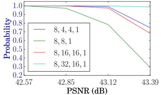
Figure 1: The probability that an ANN results in images with at least a specific PSNR value. The first (8) and last layer (1) of each ANN corresponds to the input and output layers respectively. The ANNs are listed in decreasing execution time see Figure 2 for a more detailed speedup, output quality comparison
