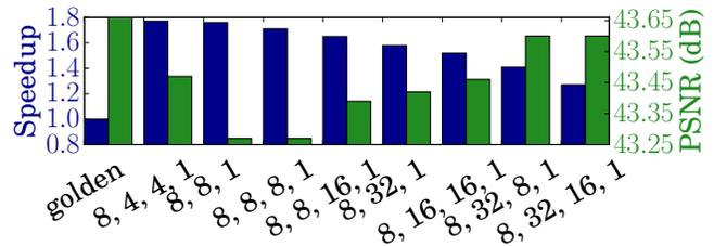
Figure 2: Speedup vs average quality comparison for the top 8 ANN topologies in terms of output quality. The X axis indicates the ANN topologies. The left Y axis shows the speedup with respect to a golden/error-free execution. The right Y axis shows the average output PSNR
