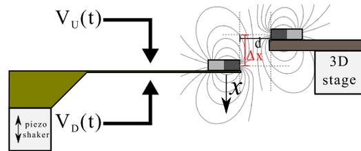
Figure 1. Schematic of the whole system and measurement setup. Lateral view of the whole system and measurement setup.
