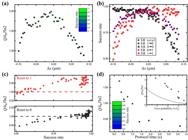
Figure 2. Produced heat and probability of success for the reset operation. (a) Average heat produced during the reset operation as function of the vertical alignment  $\Delta x$ . (b) Success rate of the reset operation as function of vertical alignment. (c) Relation between success rate and heat dissipated. (d) Dependence of  $Q$  with the protocol time duration,  $\tau_p$ . [11]
